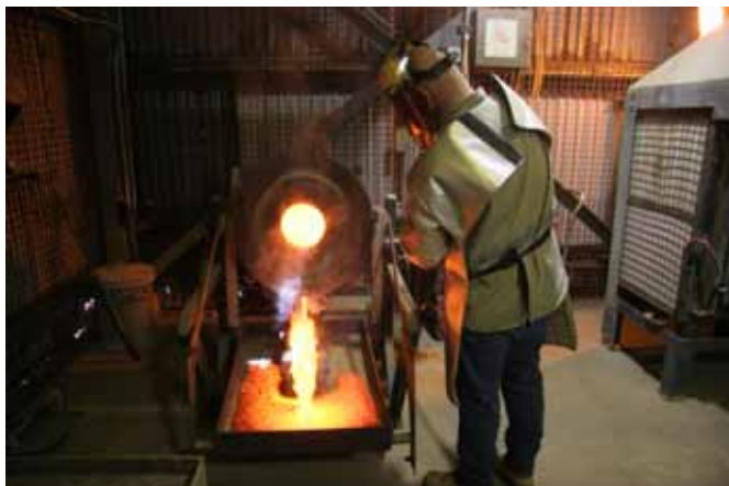
GBS Gold pours bars of their product at their Union Reef processing plant.
