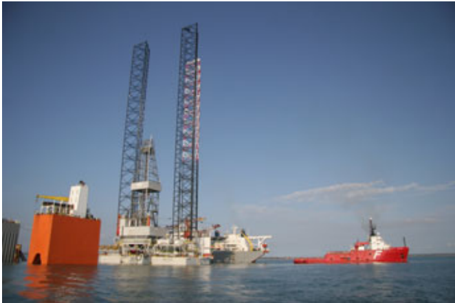
MEO Australia's West Atlas drilling rig is launched from the heavy transport vessel, Blue Marlin.
