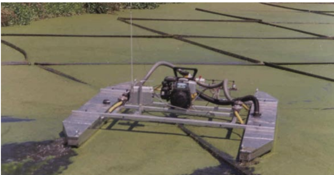
Photo 2. Remote controlled and venturi propelled mechanical duckweed harvester by Bio-Tech Waste Management (photo courtesy Robert Bell).
